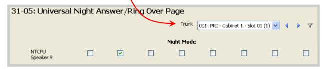
In this example the **Speaker 9** (audio out of side of cabinet or front of CP00) will supply ringing tone to an external amplifier or PA system on incoming calls to DID 2222. **Speaker 9** is the built in page port on the IPKII and SV8100. Other external outputs are also available (Speaker 1~8) via **PGD** adapters.
