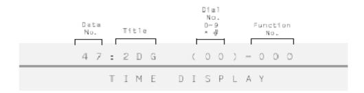
Using the \* key to scroll left and the # key to scroll right, Change the 00 after 2 DG to 79, Once you have changed 00 to 79 scroll the cursor to the 3 digit number to the right of the = sign and change that number to 148, then press TRANSFER (TRF) to save your entry.
